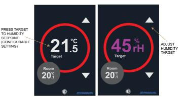
possible to adjust the humidity setpoint. The display returns automatically after approx. 10 seconds to display the temperature target.
